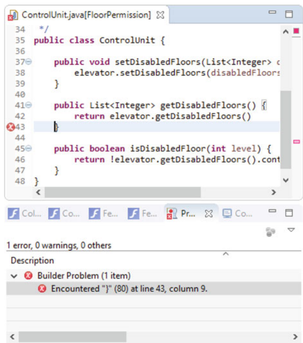
Fig. 16.2 Marker for syntax fault in feature module
