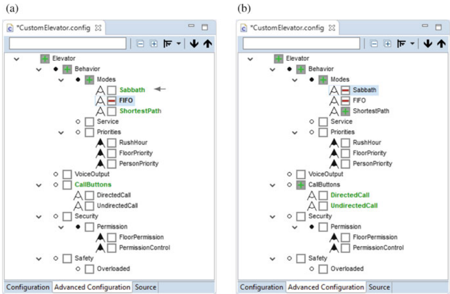
Fig. 6.5 Extended functionality of the Advanced Configuration page in the Configuration Editor. (a) Deselection of features with the Advanced Configuration editor page. (b) Automatic selections after deselection of the feature Sabbath
